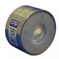
The WPCV check valve has a spring assisted poppet and a robust design suitable for a wide range of process applications. PFA, PTFE & Hastel loy to all wetted parts ensures long, high cycle performance.
