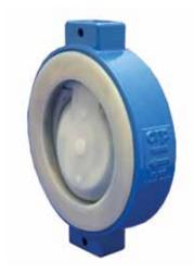
A high integrity PFA moulded wafer swing check valve, with fully encapsulated one piece disc/hinge assembly ensuring prolonged maintenance free service. Suitable for PTFE lined or unlined pipework in all severe process conditions.
